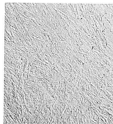
Photo 3 Electromicrograph of H.D. stress relieved Si-Cr steel wire 6 000 mag. (leplica)
