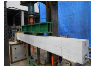
Fig. 4 Setup for loading test of a small-scale specimen
