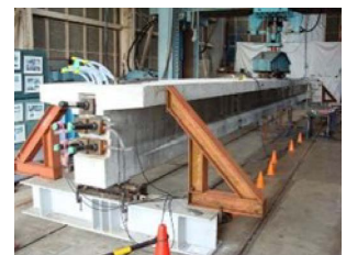
Fig. 6 Situation in loading test of full-scale specimen
